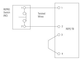
Figure 4-18. Normally-Closed REPO Switch Wiring
