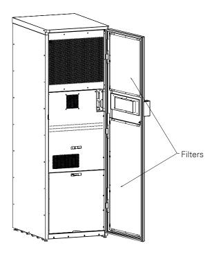
Figure 8-1. Air Filter Location
