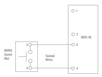
Figure 4-17. Normally-Open REPO Switch Wiring
