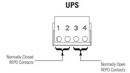
Figure 4-16. REPO Terminal Block Connector Assignments
