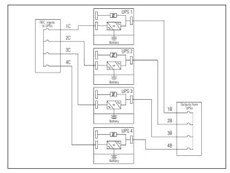
Figure 4-15. Parallel UPS system connections
