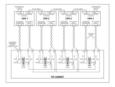
Figure 4-14. Parallel UPS Control Wiring
