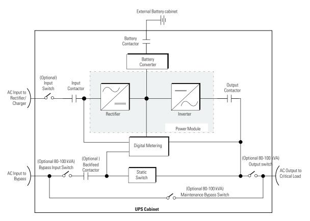
Figure 5-1. Main Elements of the UPS System
