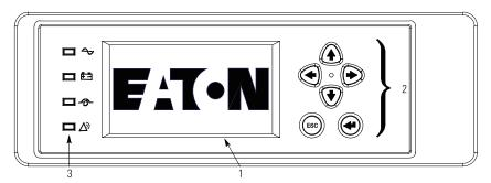
Figure 6-3. UPS Control Panel
