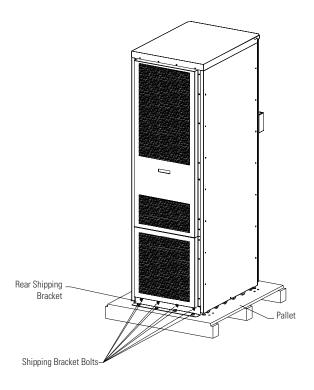
Figure 4-3. Removing the Rear Shipping Bracket
