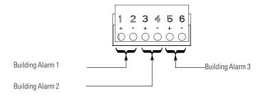
Figure 4-11. Building Alarm Terminal Block Connector Assignments
