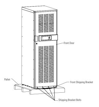
Figure 4-1. Removing the Front Shipping Bracket
