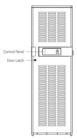
Figure 6-1. UPS Controls and Indicators
