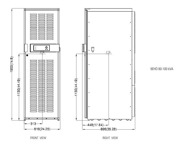
Figure 3-3. UPS Cabinet Centre of Gravity
