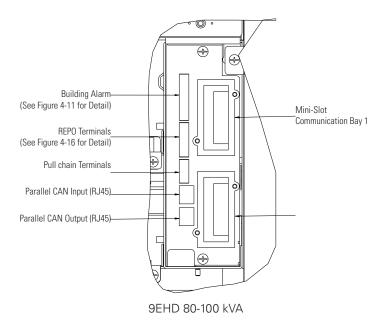
Figure 4-10. Interface Terminal Detail (Terminal Cover Removed)
