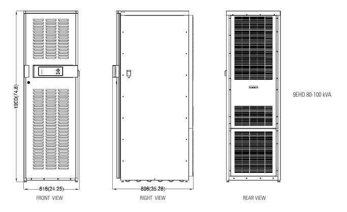
Figure 3-1. UPS Cabinet Dimensions (Front and Right Side Views)
