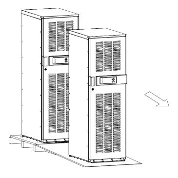
Figure 4-4. Rolling the Cabinet Down the Ramp
