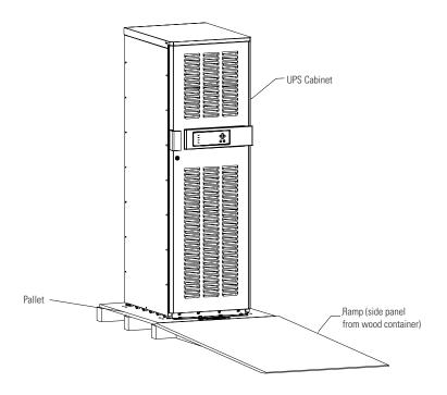
Figure 4-2. Attaching the Ramp to the Pallet
