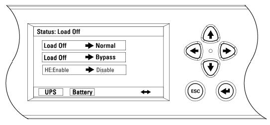
Figure 6-7. Typical System Control Screen
