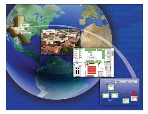
Use Layout Manager to import world and city maps, including facilities and specific gear that is monitored by the Power Xpert Software. You can design an easy drill-down user interface that also allows an alarm to bubble-up when devices trigger alarming events.
