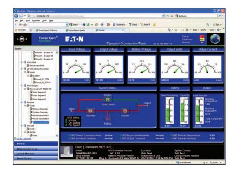
Graphic templates are built into the software for all standard Eaton devices. Viewing all of the most vital parameters along with self-explaining legends and one-line diagrams is available at a glance. Device-specific information is gathered at the bottom of the screen, including a product picture, location, system contact, maintenance schedule and asset serial number.
