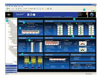
The Power Xpert Software Layout Manager module provides the user a library of powerful design tools and standard templates for the creation of custom Human–Machine Interface (HMI) graphical layouts. Objects can be easily animated, various gauges can be selected, and custom bitmaps can be imported with little effort.
