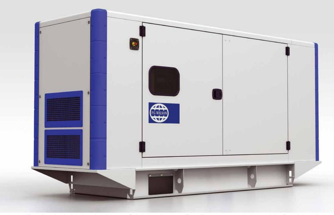
Constructed from galvanised steel with an advanced powder coat paint finish, the CAE enclosure range offers excellent protection against the elements. The base frame which extends beyond the enclosure reduces handling damage, whilst side-hinged doors enhance maintenance access and hook latches ensure operator safety by preventing unintended closure. Access for radiator cleaning and maintenance is through easily removed end panels.
