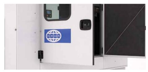
Cable access is gained directly underneath the control panel via the end of the base frame for ease of installation.
