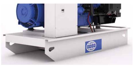
Providing lifting points as standard, aiding transportation and installation, the compact tank base is designed for 8 hours running at full load in prime applications.
