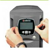
2. ROTATE THE DISPLAY PANEL COUNTER CLOCKWISE AND THEN SECURE IT BACK IN PLACE
